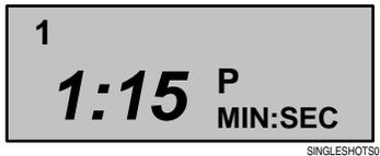
The screen above indicates that you are in Program Mode, in the Delay Time Menu and have a Delay Time set for 1 minute and 15 seconds.
